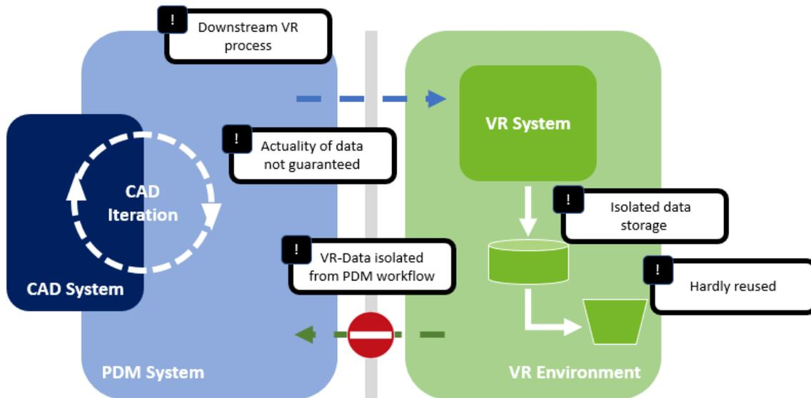
Figure 2: bidirectional data interaction between VR/AR tools and PDM systems is impossible
